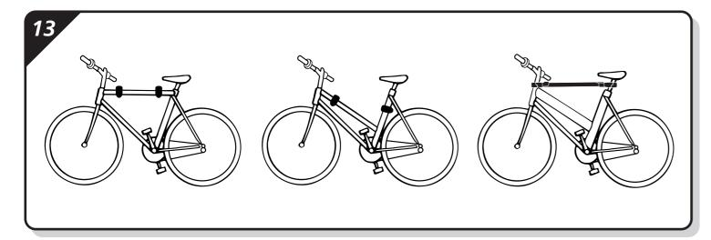
The cycle frame locators can be adjusted to best suit the angle of ladies' and children's etc, cycle frames. A FALSE cross bar is available, for the easy mounting of full suspension and low cross bar cycle frames.
